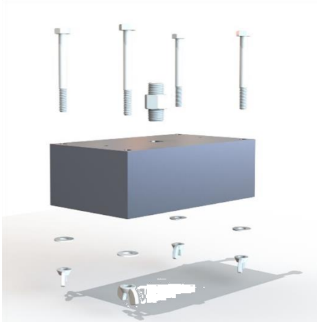
Figure 9. Full mold assembly exploded view.
