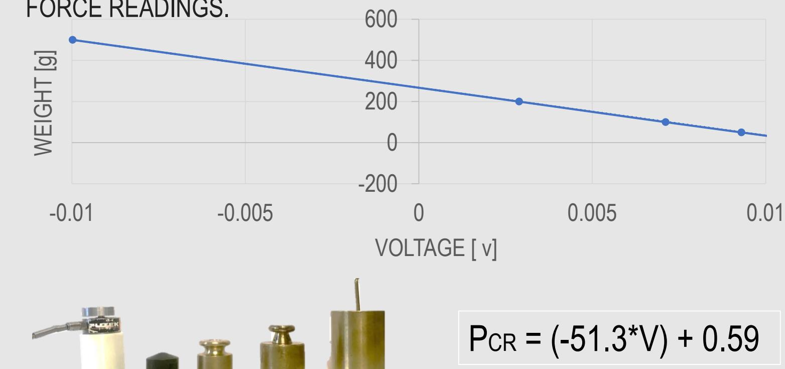
THE CALIBRATION WAS DONE WITH FIVE VARIOUS WEIGHTS. A LINE OF BEST FIT WAS DERIVED FROM THE DATA TO CREATE THE CALIBRATION CURVE.
