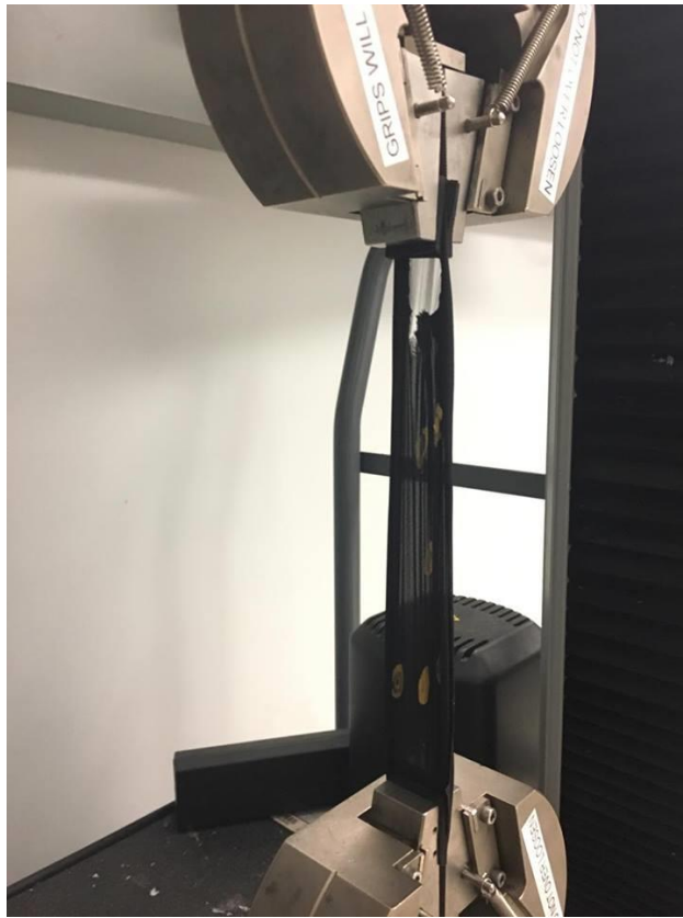
Figure 5 - material in testing apparatus experiencing failure
